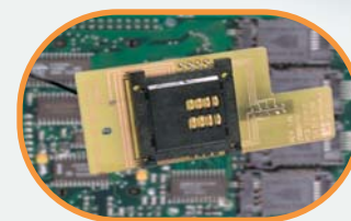
Integrated contact and contactless smart card encoding kit
